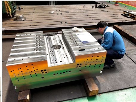
Visual inspection of cooling holes after deep drilling
