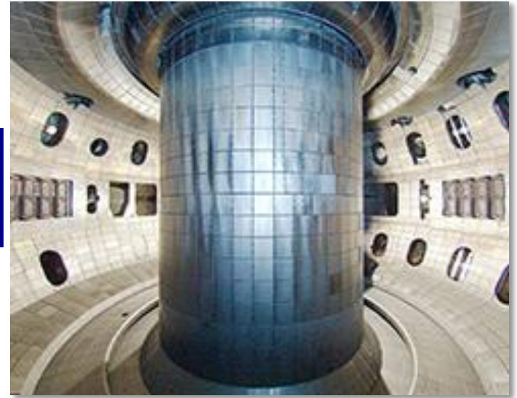
DIII-D: Largest tokamak in the U.S. Magnetic fields confine the gases
