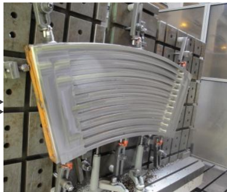
Machining leaving >5mm over-metal
