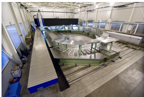
Final machining with portal machine based on DP trajectory
