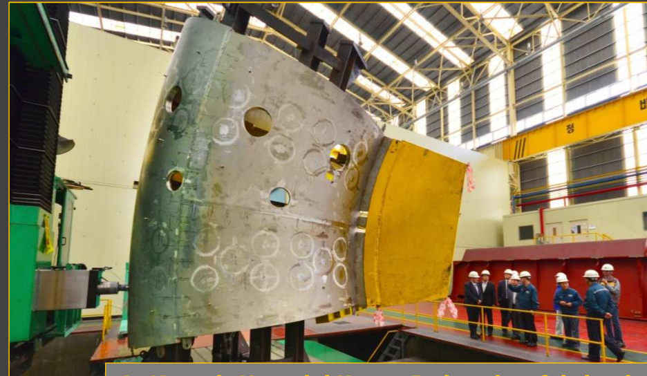
At Korea's Hyundai Heavy Industries, fabrication of 2 vacuum vessel sectors is ongoing.
